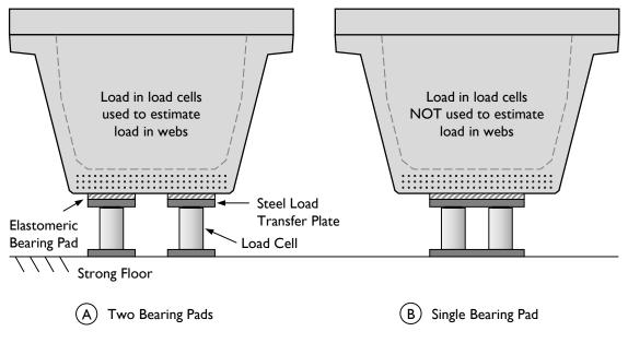
Figure 6-12: Bearing conditions used in U-Beam load tests.
