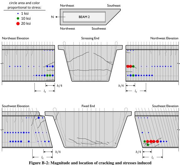
Beam 2: End-Region Stresses and Cracking at Prestress Transfer
