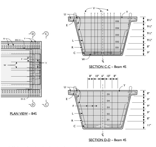
Figure A-23: Beam 4 south end region plan views and cross-sections.
