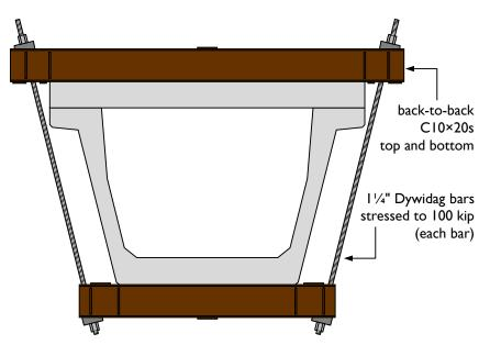
Figure 3-19: External post-tensioning system used to strengthen U-Beams during shear testing.
