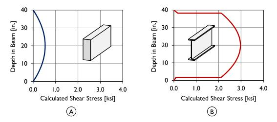
Figure 7-8: Example calculations for shear stress using (A) rectangular and (B) I-shaped beams.
