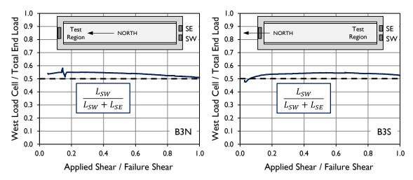
Figure B-12: Distribution of load into two bearing pads during testing of specimens B3N and B3S.
