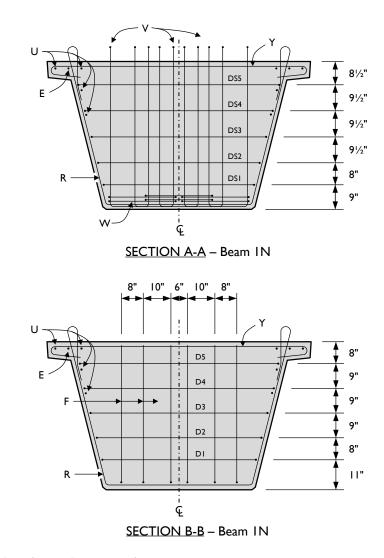
Figure A-9: Beam 1 north end-region plan view and cross-sections.
