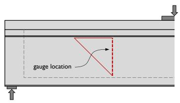
Figure B-33: Location of linear potentiometer used to measure vertical strain during loading.
