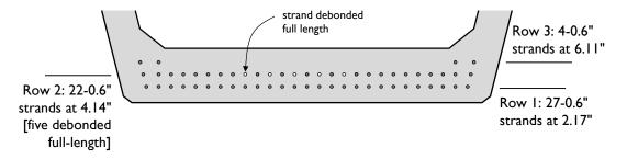
Figure A-33: Prestressing strand positions for Beam 7.
