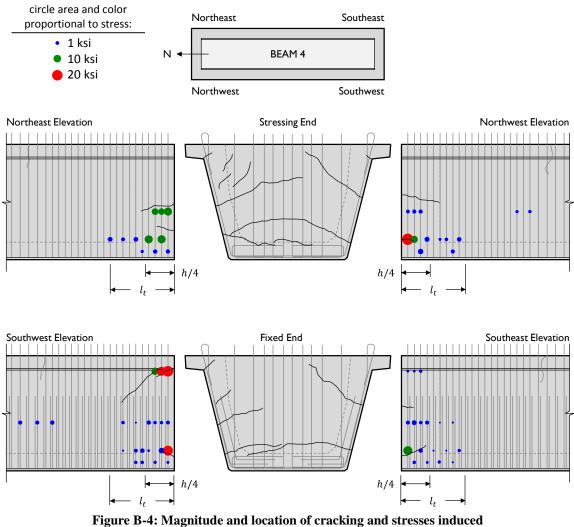
Beam 4: End-Region Stresses and Cracking at Prestress Transfer
