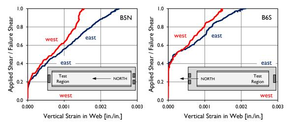
Figure B-36: Vertical strains measured in the webs of test specimens B5N and B6S during loading.
