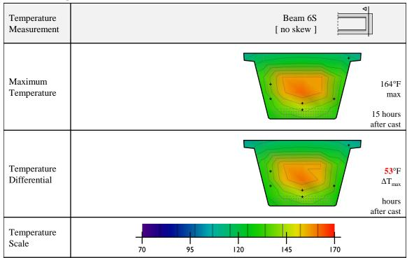
Table B-5: Temperature measurements in Beam 6 (cast November, 2010).
