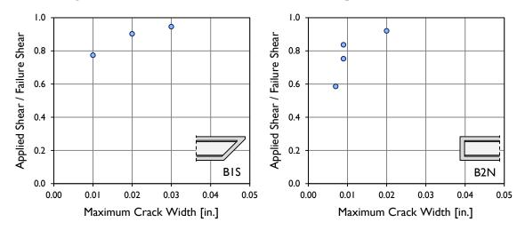
Figure B-28:Maximum crack widths measured in test specimens B1S and B2N.
