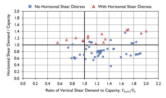
Figure 7-23: Ratios of vertical and horizontal shear demand to capacity for specimens in the HSED.
