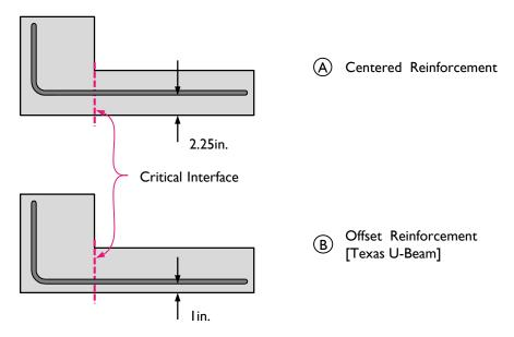
Figure 7-32: Placement of reinforcing bars crossing critical plane in modified push-off specimens.
