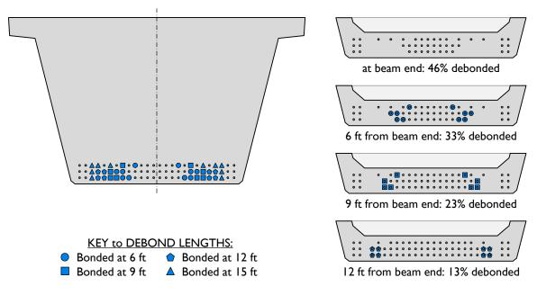
Figure 4-8: Debonding pattern for Beam 3.
