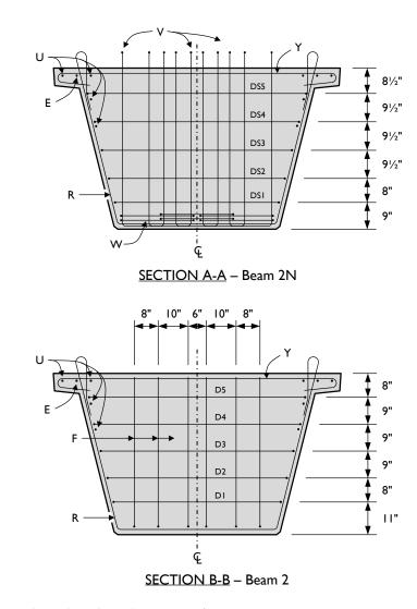
Figure A-13: Beam 2 north end-region plan view and north and south cross-sections.
