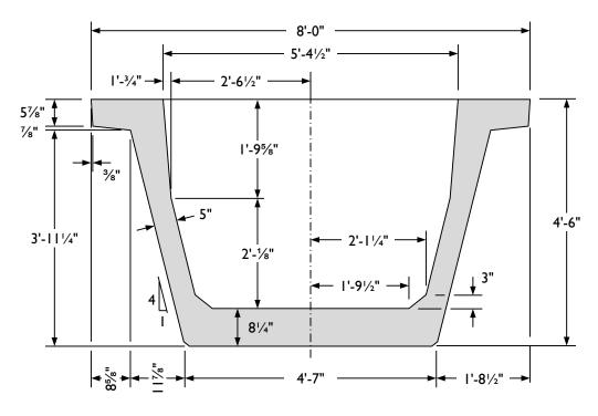
Figure 3-2: Geometry of the Texas U54 beam.
