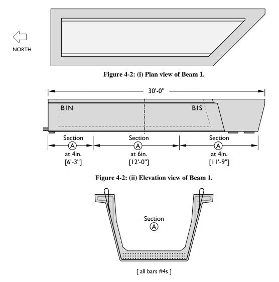
Figure 4-2: (iii) Standard cross section of Beam 1.
