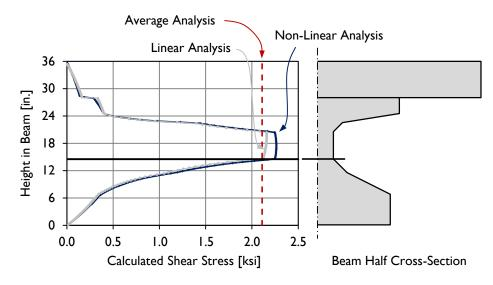
Figure 7-12: Calculated shear stress in the example Tx28, using non-linear and linear sectional analyses, and an average shear stress calculation.
