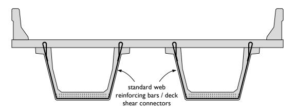
Figure 2-2: Cross section of U-Beam bridge, with standard web reinforcing bars highlighted.
