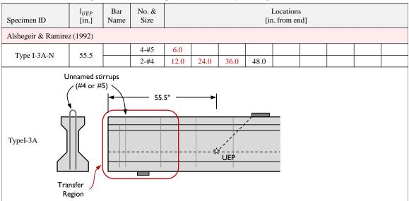
Table C-5: Reinforcing bar locations in specimens tested by Alshegeir and Ramirez (1992) (3 of 3).
