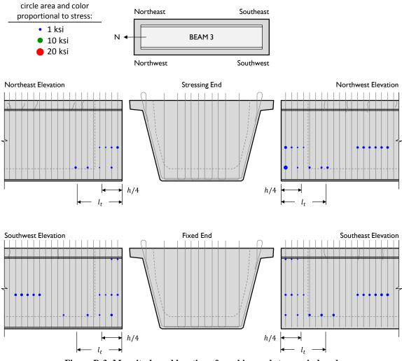
Beam 3: End-Region Stresses and Cracking at Prestress Transfer
