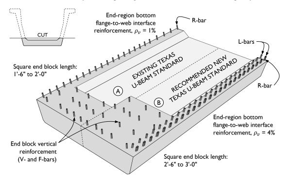
Figure 8-3: (A) Existing bottom flange-to-web interface reinforcement and (B) recommended new reinforcement.
