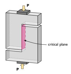
Figure 7-26: Typical push-off specimen as described in literature.
