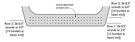
Figure A-15: Prestressing strand positions for Beam 3.
