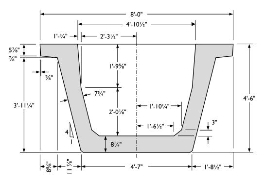
Figure A-24: Cross-sectional dimensions of the modified U-Beam used in Beam 4.
