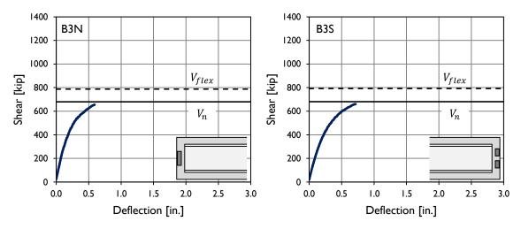
Figure B-47: Shear-deflection plot for specimens B3N and B3S.
