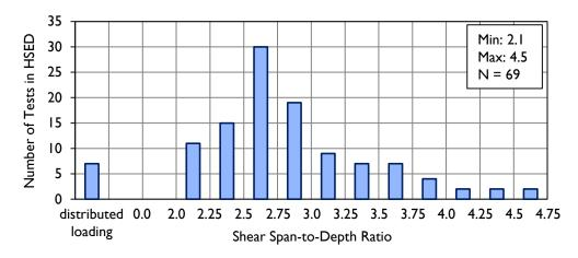
Figure 7-21: Distribution of shear span-to-depth ratio used in tests in the HSED.
