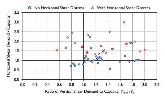
Figure 7-24: HSR-SPR plot for specimens in the HSED with calculations for capacity performed using the ACI (2008) shear-friction equation.
