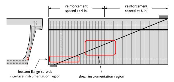
Figure 6-24: Locations of gauges monitored during shear testing.
