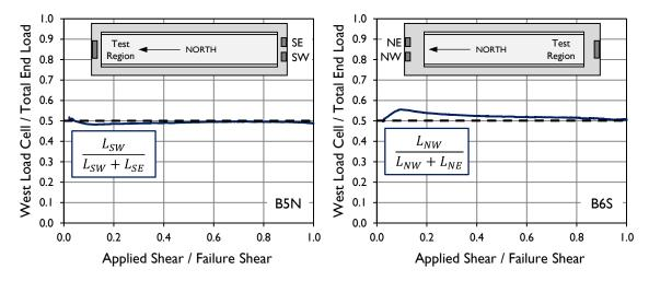
Figure B-14: Distribution of load into two bearing pads during testing of specimens B5N and B6S.
