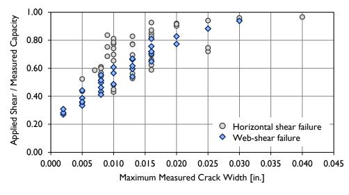
Figure 6-14: Maximum measured crack width plotted against the ratio of applied shear to failure shear.
