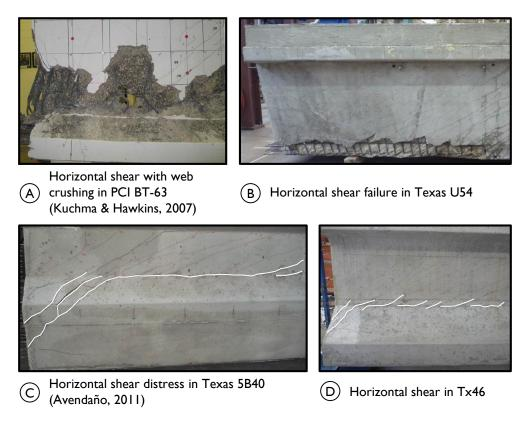
Figure 7-1: Examples of horizontal shear damage observed in laboratory tests.
