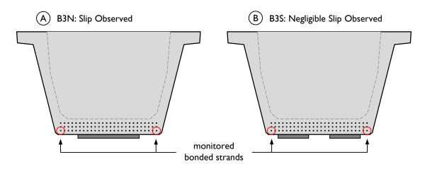
Figure 6-23: Bearing condition and monitored strand locations for B3N and B3S.
