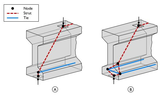
Figure 2-15: Strut-and-tie model for beam with (A) fully bonded tendons and (B) significant numbers of unbounded tendons located beneath the web (from Hamilton, Llanos, and Ross, 2009).
