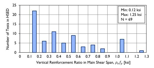
Figure 7-22: Distribution of vertical reinforcement ratio for specimens in the HSED.
