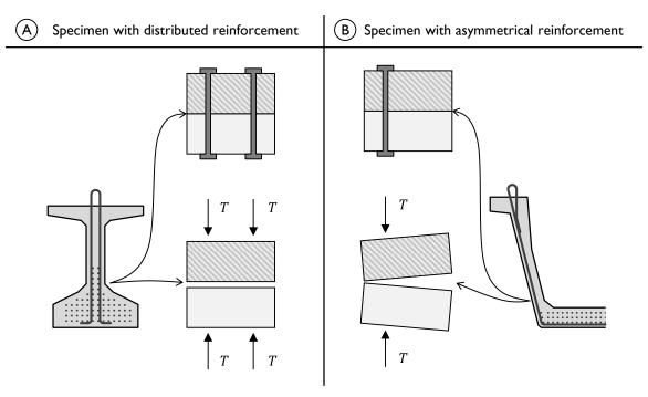
Figure 7-34: Cross-sectional view of shear-friction specimens with (A) distributed and (B) asymmetrical reinforcement.
