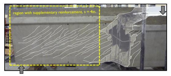
Figure 5-8: Test region B5N after flexure-shear failure.
