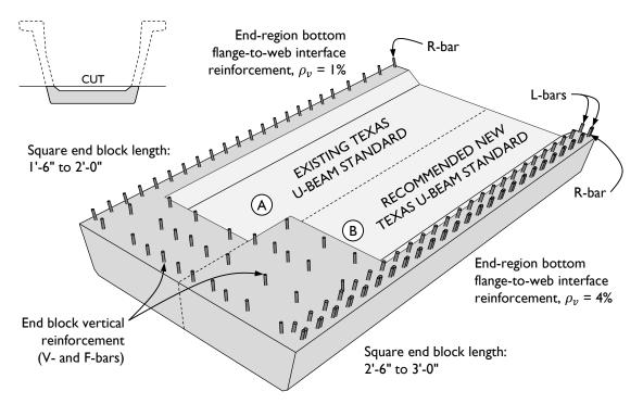
Figure 6-37: Sectional view of (A) the existing U-Beam standard and (B) the recommended new U-Beam standard, highlighting added reinforcement and increased end block length.
