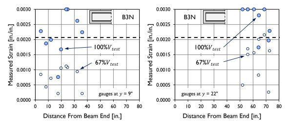
Figure B-40: Strain measured in reinforcing bars during load-testing of specimen B3N.
