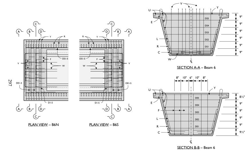
Figure A-32: Beam 6 end-region plan views and cross-sections (1 of 2).
