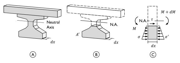
Figure 7-7: (A) Representative slice of beam, (B) considering only the area beneath the plane of interest (shaded), (C) stress resulting from the applied load.
