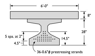
Figure 7-14: Cross-sectional properties of the example Tx28-I-D specimen.
