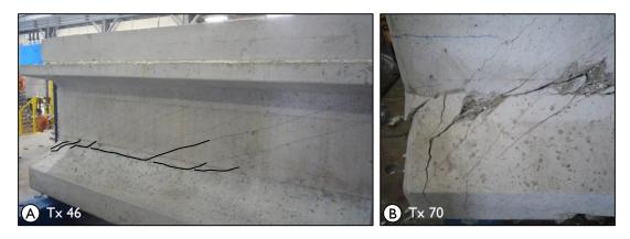
Figure 2-17: Horizontal shear damage visible in specimens (A) Tx46-S and (B) Tx70-N.
