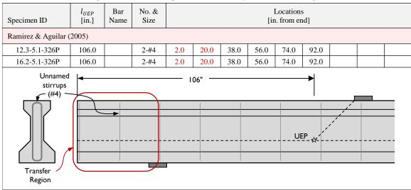
Table C-14: Reinforcing bar locations in specimens tested by Ramirez and Aguilar (2005).
