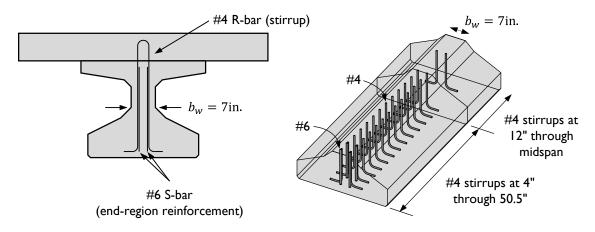
Figure 7-16: Reinforcing bar layout in specimen Tx28-I-D.
