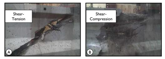
Figure 7-2: Examples of typical web-shear failures (from Heckmann and Bayrak, 2008).
