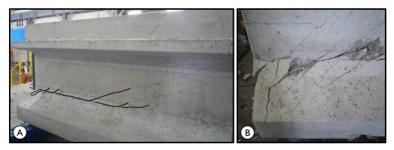
Figure 7-3: Example of horizontal shear failure.
