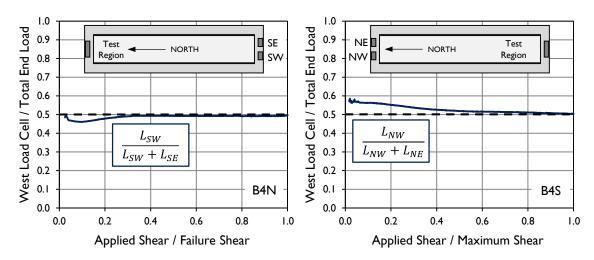
Figure B-13: Distribution of load into two bearing pads during testing of specimens B4N and B4S.
