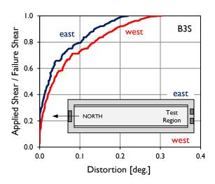
Figure B-5: Distortion measured in the webs during loading of test specimen B3S.
