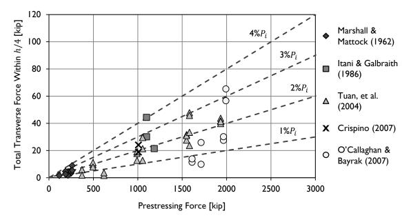
Figure 2-11: Total transverse-bar force within h/4 vs. prestressing force measured in previous beam tests from the literature (from Dunkman (2009)).
