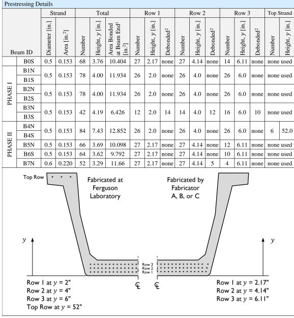
Table 3-7: Details of prestressing used in U-Beam test specimens.
