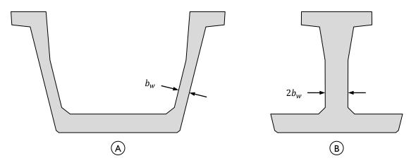
Figure 6-8: (A) Actual shape of a Texas U-Beam and (B) effective shape for calculations.
