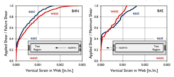
Figure B-35: Vertical strains measured in the webs of test specimens B4N and B4S during loading.
