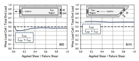
Figure B-10: Distribution of load into two bearing pads during testing of specimens B0S and B1N.
