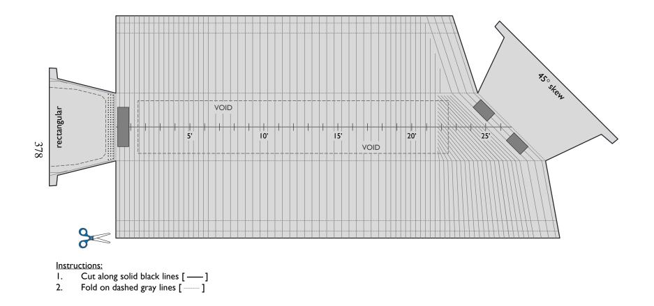
Figure E-1: Model of 30-ft Texas U54 with detailing matching current standard.
