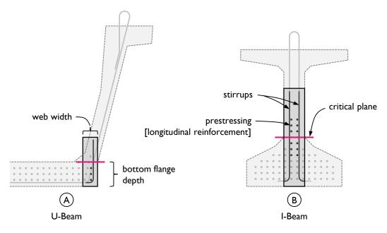
Figure 7-28: Critical interface of push-off specimens based on the reinforcement of (A) a standard Texas U-Beam and (B) an I-Beam (Tx 46).
