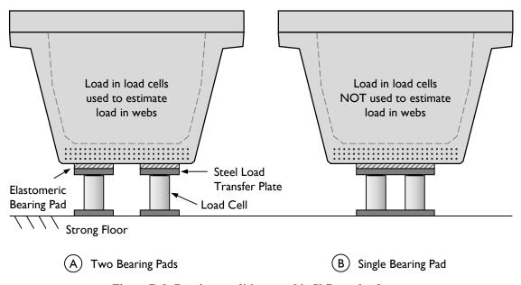
Figure B-9: Bearing conditions used in U-Beam load tests.
