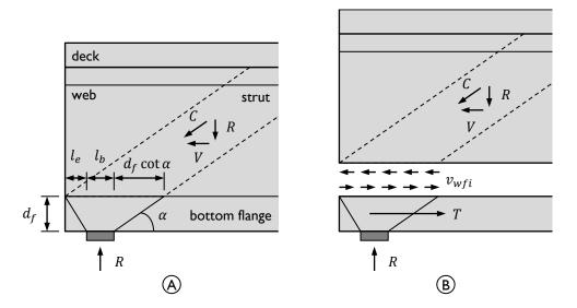
Figure 2-14: End region of the beam model used by Nagle and Kuchma (2007) showing (A) dimension definitions and (B) location of horizontal shear stress.
