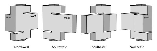
Figure 7-31: Modified push-off specimen viewed from four corners.
