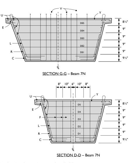
Figure A-36: Beam 7 north end-region plan views and cross-sections (2 of 2).
