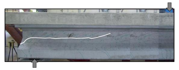
Figure 7-17: Tx28-I-D cracking observed at failure.
