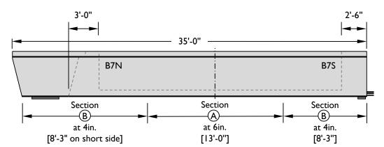
Figure 5-16: (ii) Elevation view of Beam 7.
