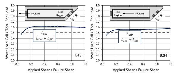
Figure B-11: Distribution of load into two bearing pads during testing of specimens B1S and B2N.
