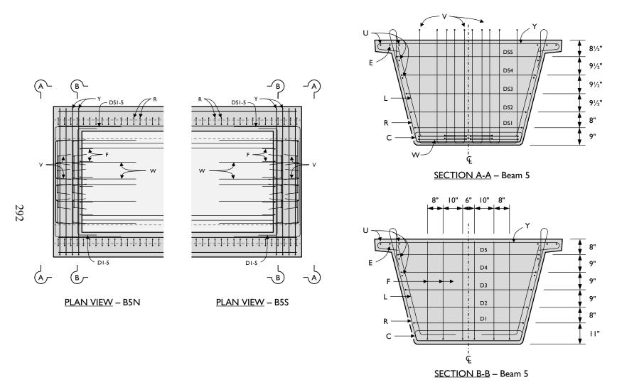
Figure A-28: Beam 5 end-region plan views and cross-sections.
