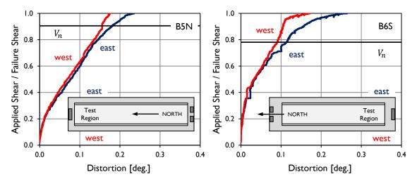
Figure B-7: Distortion measured in the webs during loading of test specimens B5N and B6S.
