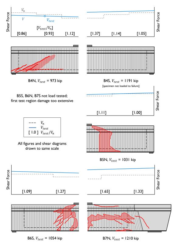
Figure 6-31: Summary of Phase II U-Beam shear tests.
