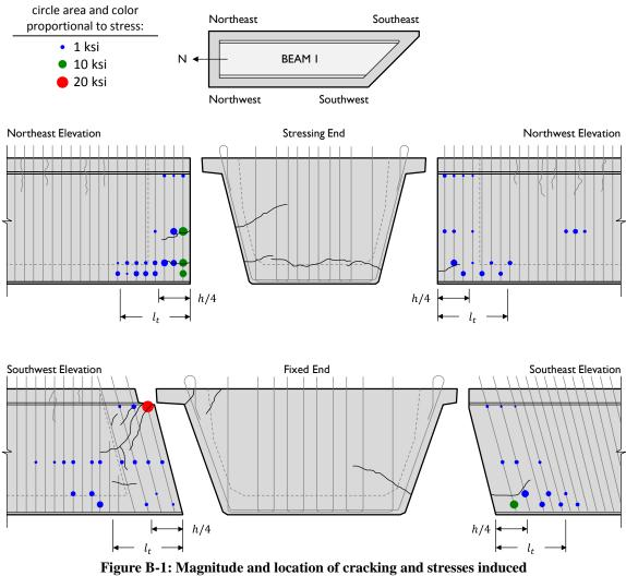
Beam I: End-Region Stresses and Cracking at Prestress Transfer
