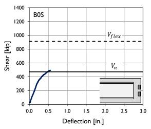
Figure B-44: Shear-deflection plot for specimen B0S.
