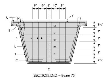
Figure A-37: Beam 7 south end-region plan views and cross-sections (2 of 2).
