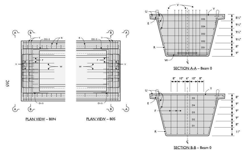
Figure A-6: Beam 0 end-region plan views and cross-sections.
