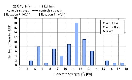
Figure 7-19: Distribution of concrete strength for specimens in the HSED.
