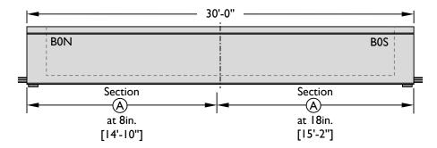
Figure 4-1: (i) Beam 0 elevation view, with reinforcing bar spacings indicated.
