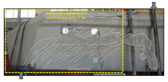
Figure 5-17: Test region B7N after shear failure.
