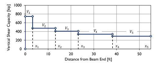
Figure 7-38: Typical vertical shear capacity plot.
