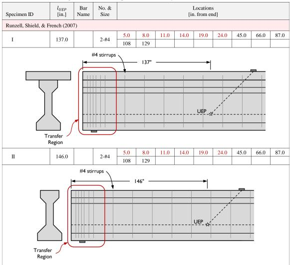
Table C-15: Reinforcing bar locations in specimens tested by Runzell, Shield, and French (2007).
