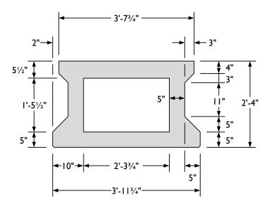
Figure 2-18: Cross-sectional dimensions of the Texas 4B28 tested by Avendaño (2011).
