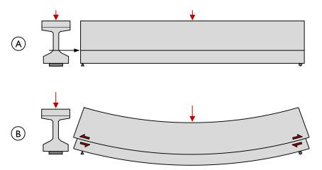
Figure 7-5: Horizontal shear schematic.
