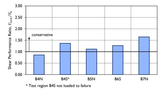
Figure 5-18: Ratio of failure shear to calculated shear capacity for the five Phase II test specimens.
