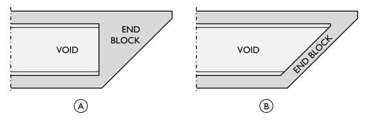
Figure 3-3: Plan view of end block options in skewed U-Beams: (A) square void with triangular end block, and (B) skewed void with square end block.
