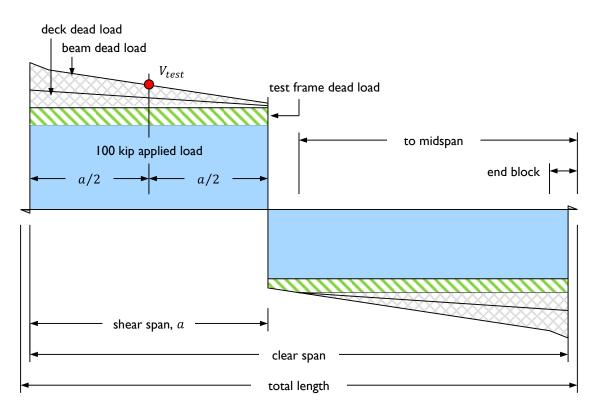
Figure 3-22: Explanation of the location and magnitude of V<sub>test</sub>.
