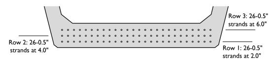
Figure A-7: Prestressing strand positions for Beam 1.
