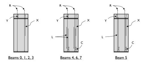
Figure A-3: Key showing reinforcing bar appearance in elevation view.
