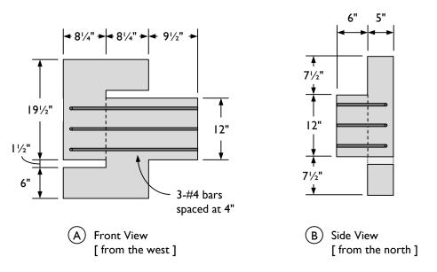
Figure 7-30: Dimensions and interface reinforcing bar locations in modified push-off specimens.
