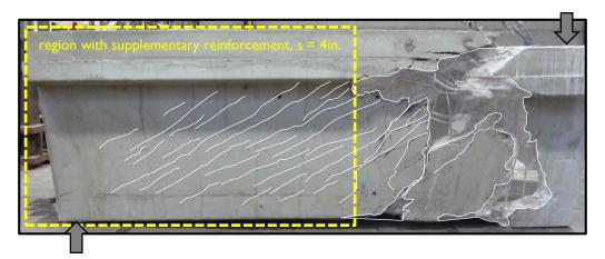
Figure 5-15: Test region B6S after flexure-shear failure.
