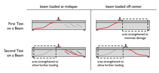
Figure 3-20: Schematic of how and when external post-tensioned clamps were used to aid in achieving a second failure within one beam.
