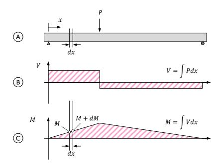
Figure 7-6: (A) Example beam, (B) shear diagram, and (C) moment diagram.
