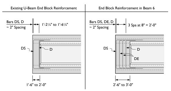
Figure 5-14: Existing end block reinforcement compared with reinforcement used in Beam 6.
