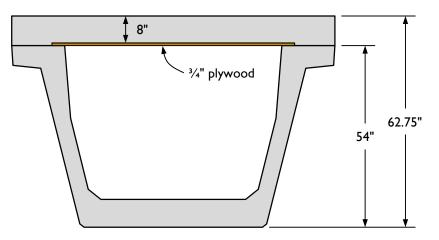
Figure 3-15: Deck form system used, highlighting <sup>3</sup>/<sub>4</sub>" plywood.
