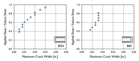
Figure B-31: Maximum crack widths measured in test specimens B5N and B6S.
