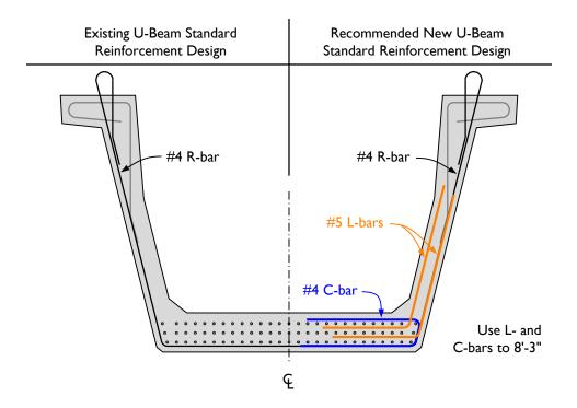
Figure 8-1: Existing and recommended U-Beam standard reinforcement.
