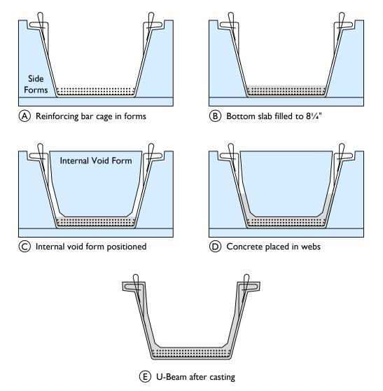
Figure 3-10: Two-stage monolithic cast procedure.
