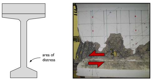
Figure 2-13: Horizontal sliding failure mode seen in several of the BT-63 specimens tested by Nagle and Kuchma (2007).
