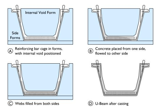
Figure 3-11: Monolithic cast procedure.
