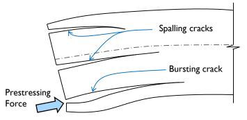
Figure 2-10: Bursting and spalling deformations (from Dunkman 2009).
