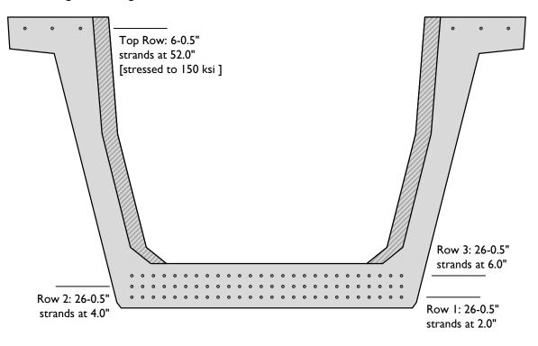
Figure A-19: Prestressing strand positions for Beam 4.
