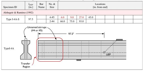
Table C-5: Reinforcing bar locations in specimens tested by Alshegeir and Ramirez (1992) (2 of 3).
