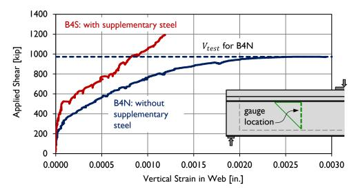
Figure 6-17: Vertical strain measured through the webs of Beam 4.
