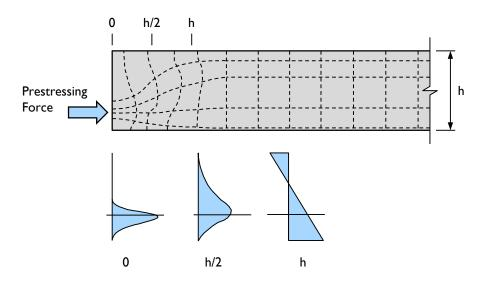
Figure 2-9: Spreading of near anchorage zone (from Nilson (1987)).
