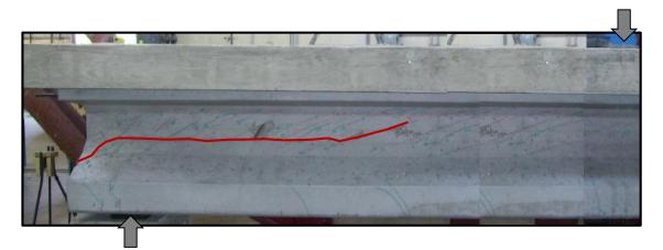
Figure 2-16: Tx28 after shear testing, with horizontal failure crack highlighted.
