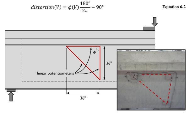
Figure 6-9: Linear potentiometers locations on web, for measuring distortion.
