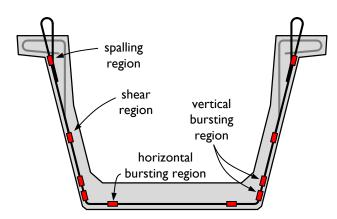
Figure 3-13: Location of instrumentation monitored at prestress transfer.
