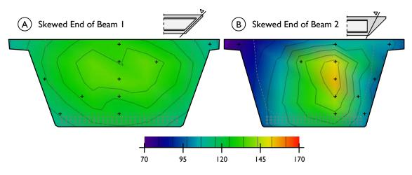
Figure 6-7: Temperatures measured through the cross sections of the skewed end blocks of Beam 1 and Beam 2 at time of maximum temperature reading.
