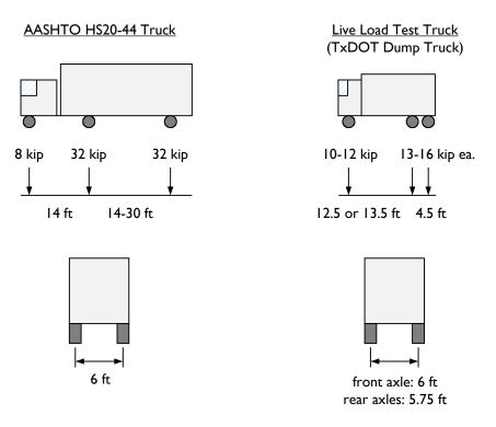
Figure 2-7: Live loading scheme used by Gross and Burns (2000).
