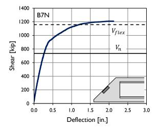
Figure B-50: Shear-deflection plot for specimens B7N.
