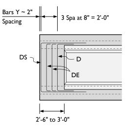
Figure 6-36: Reinforcing bar changes in the end block.
